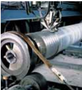
Hard-surfacing of mill rolls with strip cladding
